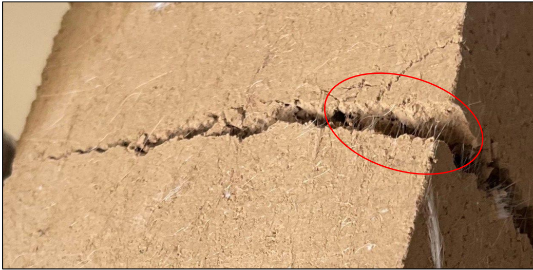
Fig. 15. Fibers bridging crack during the flexural test.
