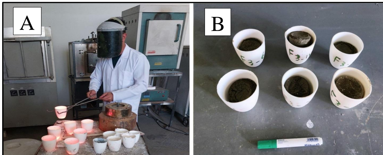
Fig. 4. A-Samples after burning, B-Clinker product.
