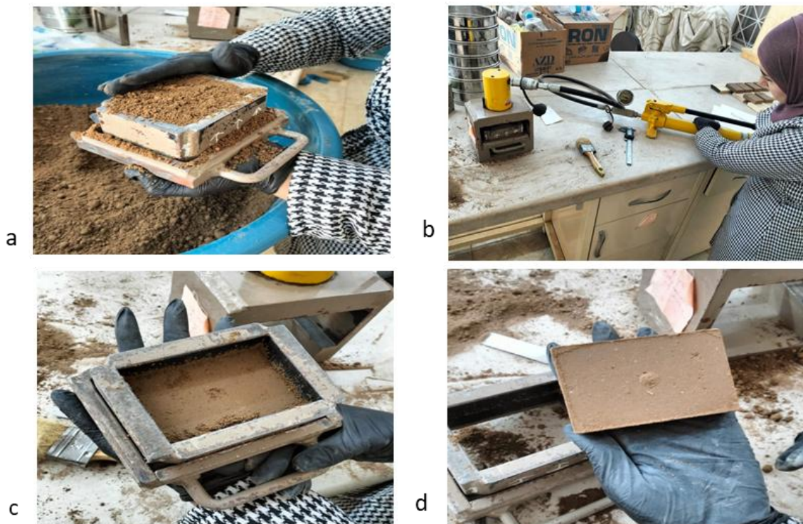
Fig. 3. The stages of production of compressed earthen bricks without and with the addition of cement.
