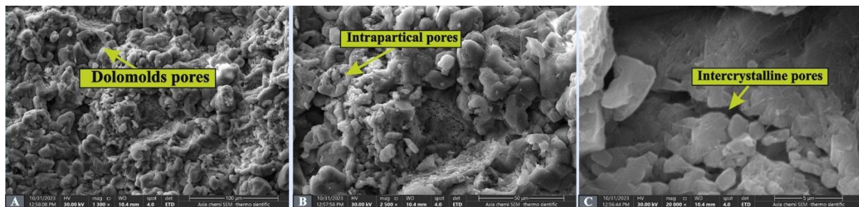
Fig. 9. SEM microphotograph showing rhomb's dolomite in crystalline dolostone; (A) Dolomolds pores; (B) Intraparticle porosity; (C) Intercrystalline porosity.
