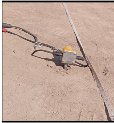
Fig. 4. Geophone (S) used in the MASW method.
